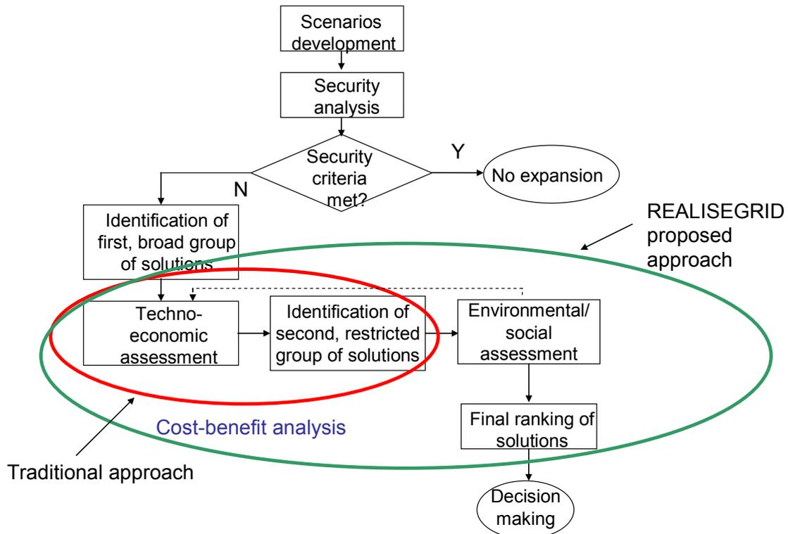
Fig 2 - Basic scheme of the transmission planning process
