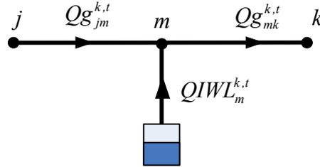
Figure 5.9: Pipeline line-pack
