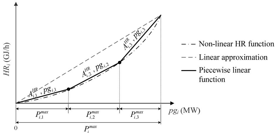
**Figure 5.3: HR piecewise linear function**
