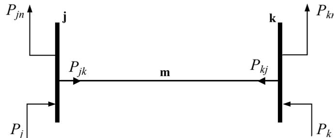
**Figure 5.5: Transmission line and active power flows**
